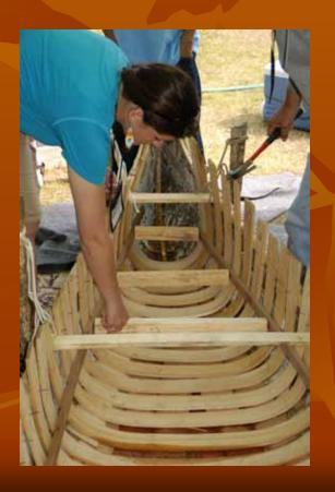
For final drying, the rough shaped and semidried ribs are carved, bundled, and numbered for proper placement in the canoe
