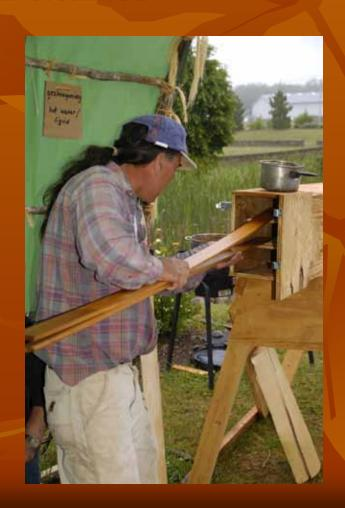
During waaginaa (canoe rib) fitting process,
