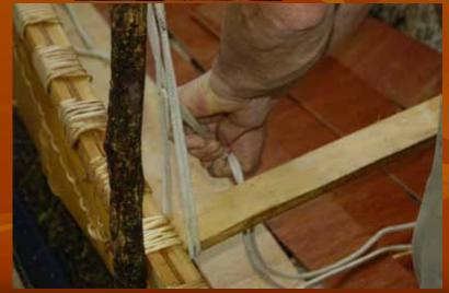
Rib wood has been soaked for several days to prepare it for steaming and fitting into canoe
