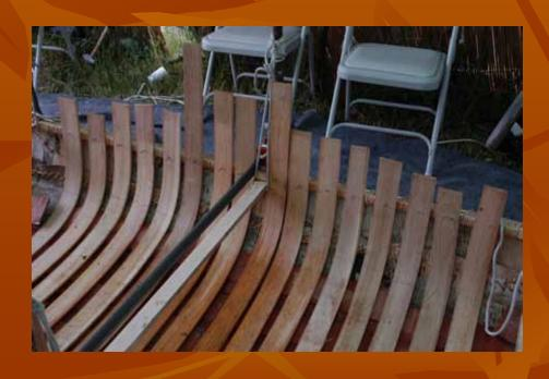
n Boards are inserted and secured to hold waaginaag (ribs) in their places while drying to their desired shape
